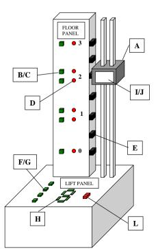
E.  $7 \times$  floor sensors (one on each floor, and one between each floor)
