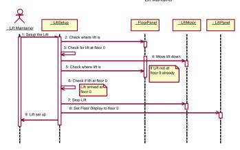
The messages shown above are then mapped to operations on the classes (see the detailed *LiftAPI* package description below for the definition of these operations). These operations are mapped to Java methods on the *LiftAPI* package classes.
