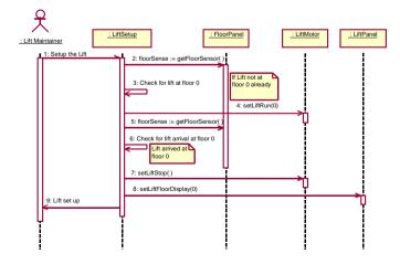
From the sequence diagram, it is clear that the *LiftSetup* class has internal state behaviour, which can be captured with a State Diagram. This behaviour is so simple that such a diagram is hardly warranted, but it serves here to illustrate a useful starting point to a larger state diagram which describes the behaviour of the *LiftController* class (or possibly several interacting classes with their own state diagrams depending on the design).
