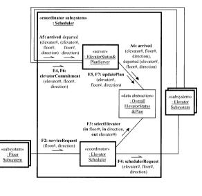
Analyse each event sequence (A, E, F) in turn for the distributed system via the Generalized Utilization Bound Theorem (GUBT)...
