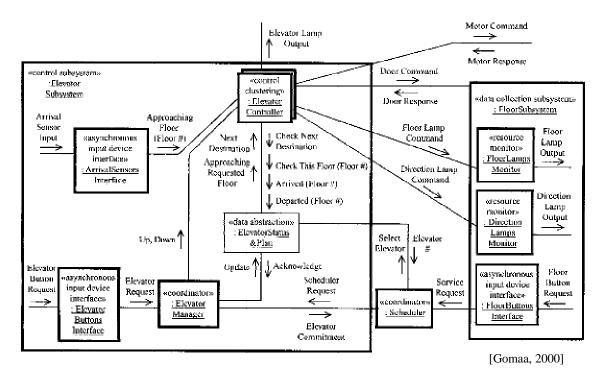
All asynchronous input device interfaces are mapped to asynchronous I/O tasks. *Elevator Manager* is designated as a coordinator task, and *Elevator Controller* is a multiple instance control task. The *Elevator Status & Plan* object is mapped to a passive data abstraction object. As the motor and door output interfaces are passive, and *Elevator Controller* must await a response, no additional I/O tasks are required to interface to these output objects.
