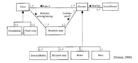
All external devices are interfaced to the system via software device interface objects so the System Context Diagram shows this mapping:
