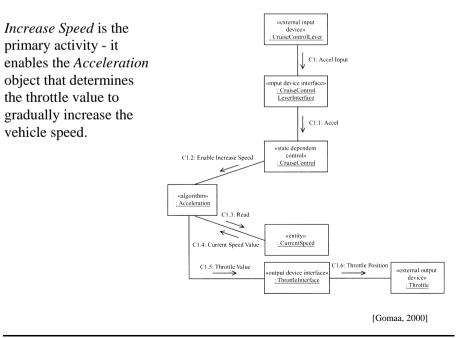
The next external event is CRUISE when the cruise control lever is released:
