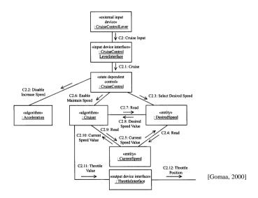
*Maintain Speed* is the primary activity - it enables the *Cruiser* object that determines the throttle value to maintain the vehicle speed.
