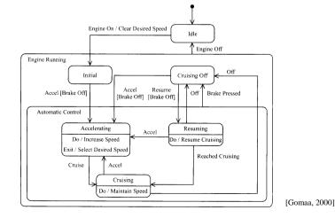
Other aspects of the *Cruise Control* object can also be modelled, e.g. the *Brake Condition* can be maintained by an additional orthogonal statechart to the Auto Cruise Control statechart already described:
