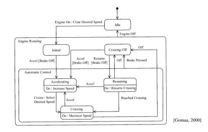
The *Brake Pressed* transition from the *Accelerating* state has a *Select Desired Speed* action  $\rightarrow$  shift to an exit action from *Accelerating*:
