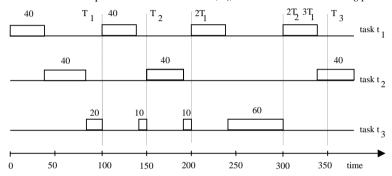
Look at the appropriate scheduling points for task 3, i.e. the ends of the periods of all higher priority tasks which have times less than or equal to task 3's period.
