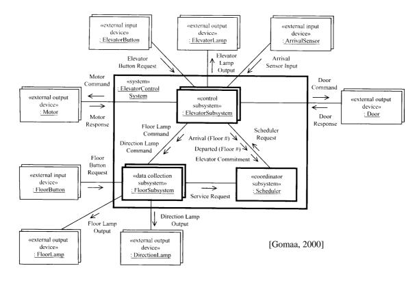
Unlike the non-distributed system, the Scheduler Subsystem and multiple instances of the Elevator Subsystem cannot communicate via shared memory, so there are two alternatives:
