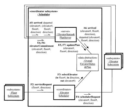
Analyse each event sequence (A, E, F) in turn for the distributed system via the Generalized Utilization Bound Theorem (GUBT)...
