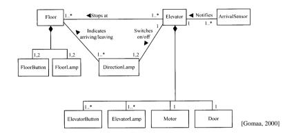
All external devices are interfaced to the system via software device interface objects so the System Context Diagram shows this mapping:
