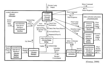
All asynchronous input device interfaces are mapped to asynchronous I/O tasks. *Elevator Manager* is designated as a coordinator task, and *Elevator Controller* is a multiple instance control task. The *Elevator Status & Plan* object is mapped to a passive data abstraction object. As the motor and door output interfaces are passive, and *Elevator Controller* must await a response, no additional I/O tasks are required to interface to these output objects.
